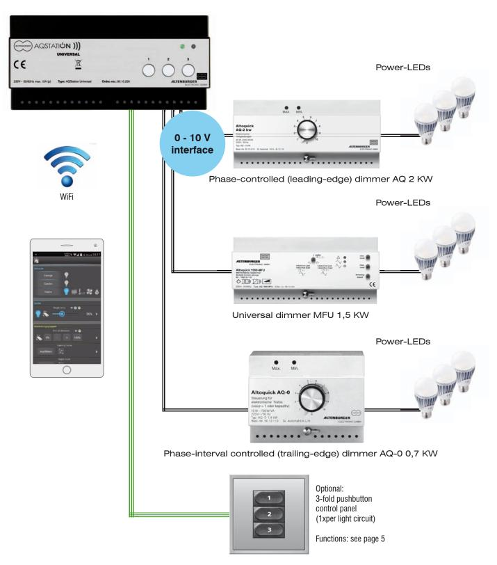
DIN rail dimmers to be combined with the AQStation Universal
