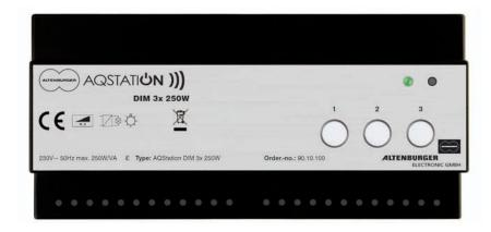
While the AQStation Universal works preferably with external load dimmers the AQStation Dim 3x 250W has 3 integrated load dimmers, operating in the phase-interval (trailing edge) mode. Each dimmer has a load capacity of 250W.
