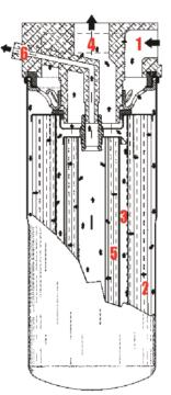
The results speak for themselves. Extensive life and efficiency tests and billions of miles of actual use prove the BD103 outperforms the LF3000. The patented "series" design and the cellulose/synthetic blend media are central to the filter's increased contaminant holding capacity and longer element life. In the BD103, all oil passes through the full-flow element instead of just part of it as with "parallel" designs. The full-flow/by-pass
