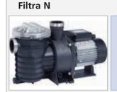
2 Q [m<sup>3</sup>/h] max. 36 H [m] max. 21 max. 2.5 p [bar] T [°C] max. +35 n [min<sup>-1</sup>] max. 2800 Recirculating pump for swimming pool filtering systems
